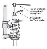
WARNING: ALWAYS USE APPROPRIATE SPRING COMPRESSOR BEFORE REMOVING TOP FIXINGS.
